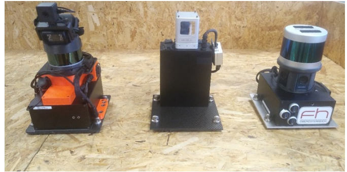
Fig. 10. Modular sensor payload system
