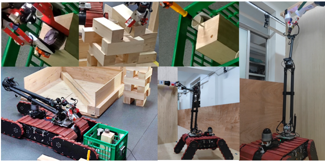
Fig. 15. Visually guided manipulator for precise operation.
