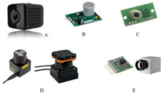
Fig. 3. Electrical components of our Robots: (A) Cameras (B) Carbon dioxide sensor (C) Heat sensor (D) Sensor Range Finder (E) Thermal sensor
