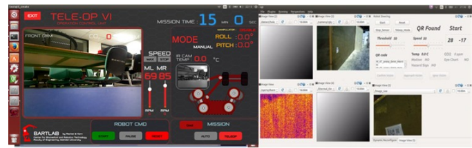
Fig. 7. Image shows the framework of (A) GUI of the tele-operative (B) GUI of the autonomous function
