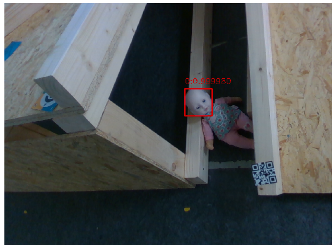
Fig. 8: Baby Doll Detection with a Realsense using YOLOv5.
