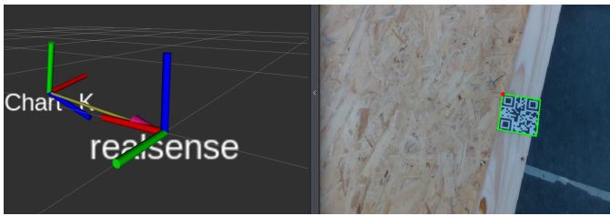
Fig. 9: Qr-Code Detection: i) In the right image, the red dot on the bounding box of the qr code denotes the top left corner of the tag. ii) In the left image, the published transformation is visualised with respect to the camera frame.
