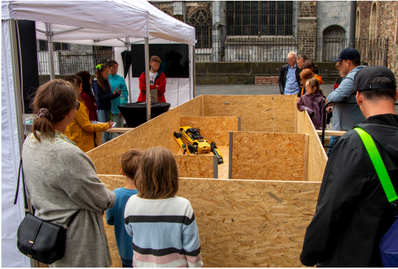
(a) Spot walks with collision avoidance through a parkour with ramps while being controlled by an operator's gestures.
