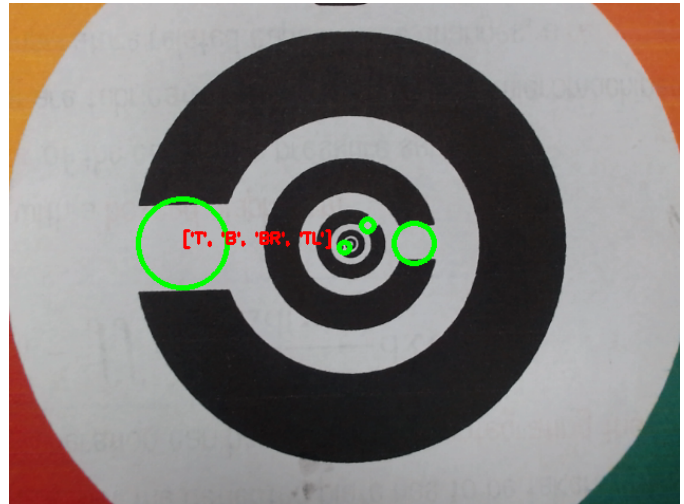
Fig. 6: Landolt Detection: The green circles in output images refer to the contour defects.
