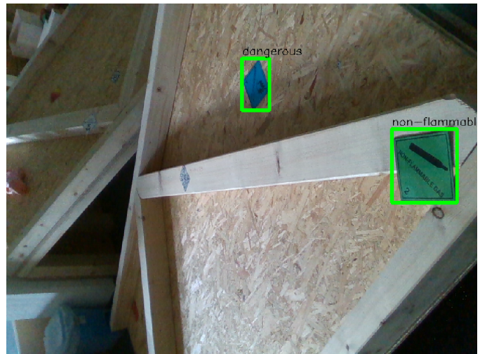
Fig. 7: Hazmat Detection of a non-flammable and dangerous sign
