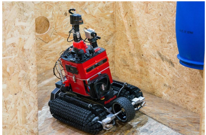
Fig. 4. Scorpion - omnidirectional rescue robot
