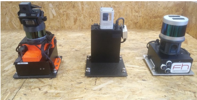
Fig. 9. Modular sensor payload system
