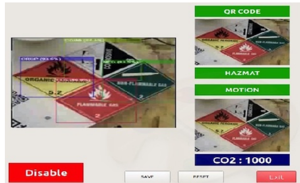
Fig. 8. The operator's display illustrated motion detection, QR code detection, and hazmat detection.
