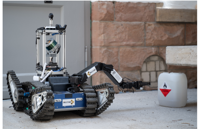
Fig. 1: Asterix rescue robot performing a visual inspection task.
