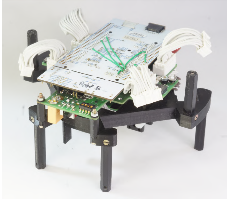
Fig. 2. 3D printed Second Floor with main board.
