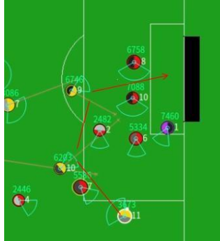
Figure 4: Best chain action is our player no.11 pass ball to no.10 and no.10 then pass ball to no.9.Then no.9 can shoot. Because of pass can be generated as the second action in chainaction and use Monte carlo tree search to find best
