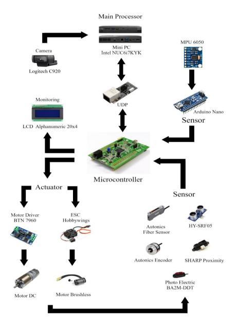
Fig. 4. Electrical System of the Robot
