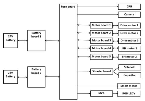
Figure 4: Robot power distribution
