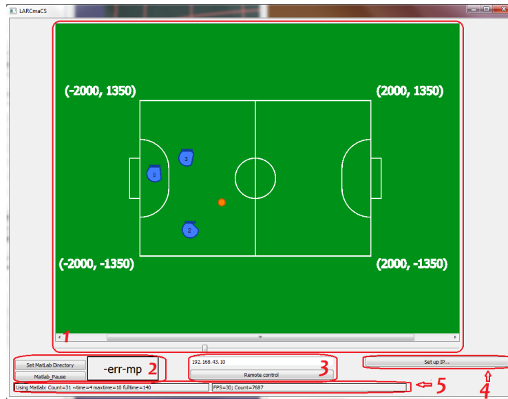
Fig. 7: Main window of our application. 1. Game Field 2. Matlab block 3. Remote control block 4. IP Settings 5. Information bars
