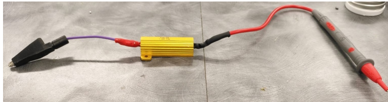
Fig. 3.1: Capacitor Discharge Circuit
