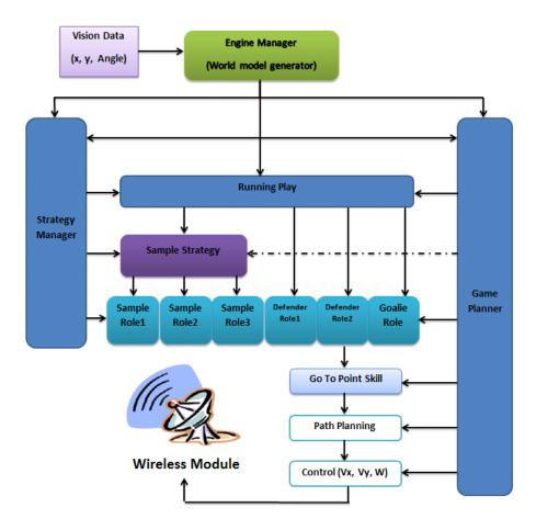
Fig. 2. Block diagram of AI structure
