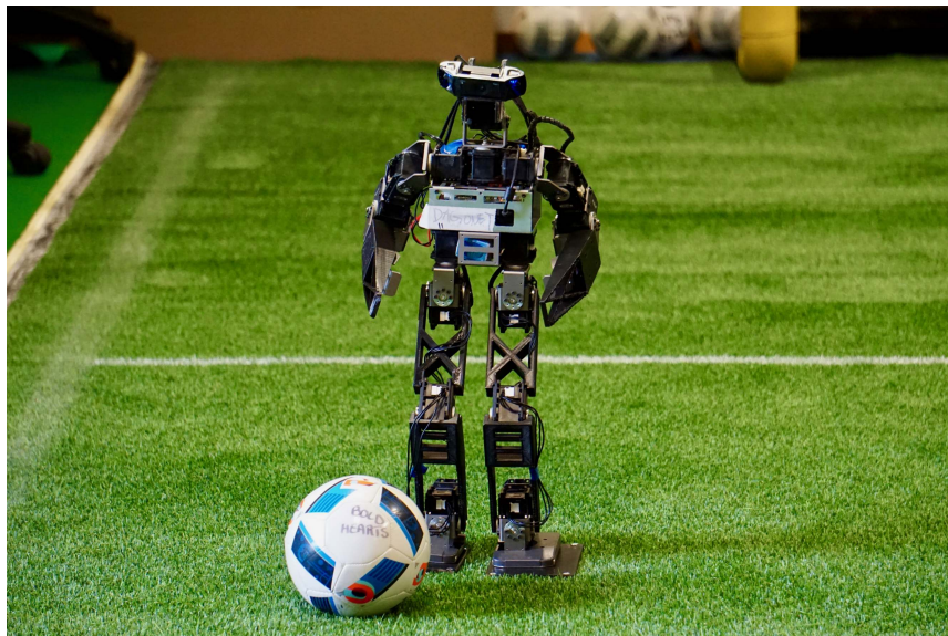
Fig. 2. The BoldBot robot in its second version. It is incrementally developed with a Darwin-OP as its base. The torso has been scaled up to fit an Odroid-XU4, the new main processing unit. The shin, thigh, arm, head bracket and the foot plate have been redesigned, scaled up and 3D printed.
