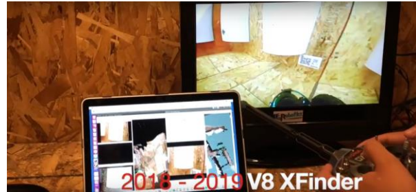
Fig.13 current operator station, going from left to right are: SLAM and 3D map, streaming video camera and robot control.
