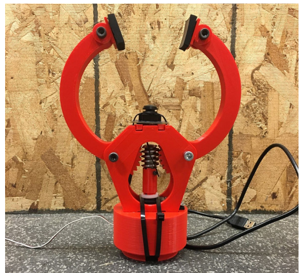
Grasper with mounted camera for object visual detection.
