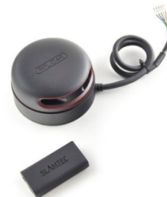
LIDAR mapping system for 3D map construction.
