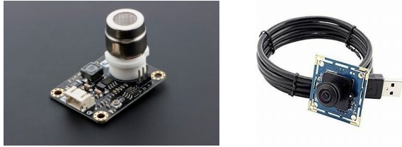
The DFRObot 0159 CO2 Sensor for life detection and the Megapixel USB Camera for image capturing.
