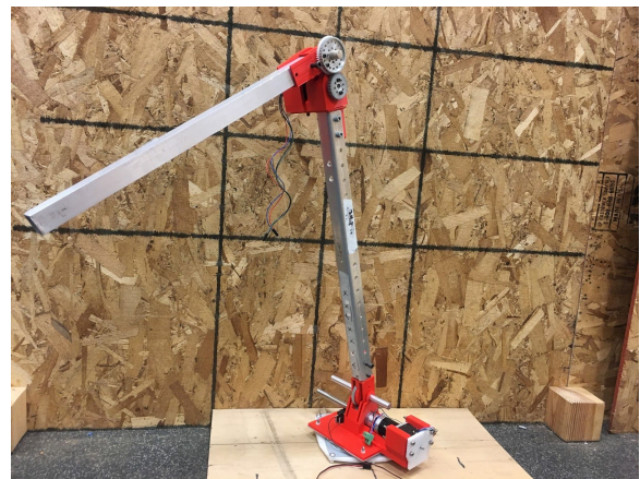
Jointed arm with rotation capabilities.
