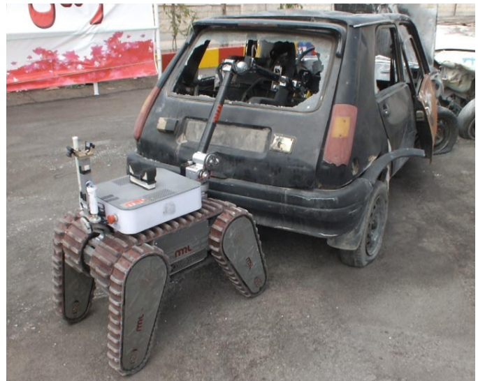
Fig. 14. Karo is inspecting inside a car using the 6-DOF manipulator.
