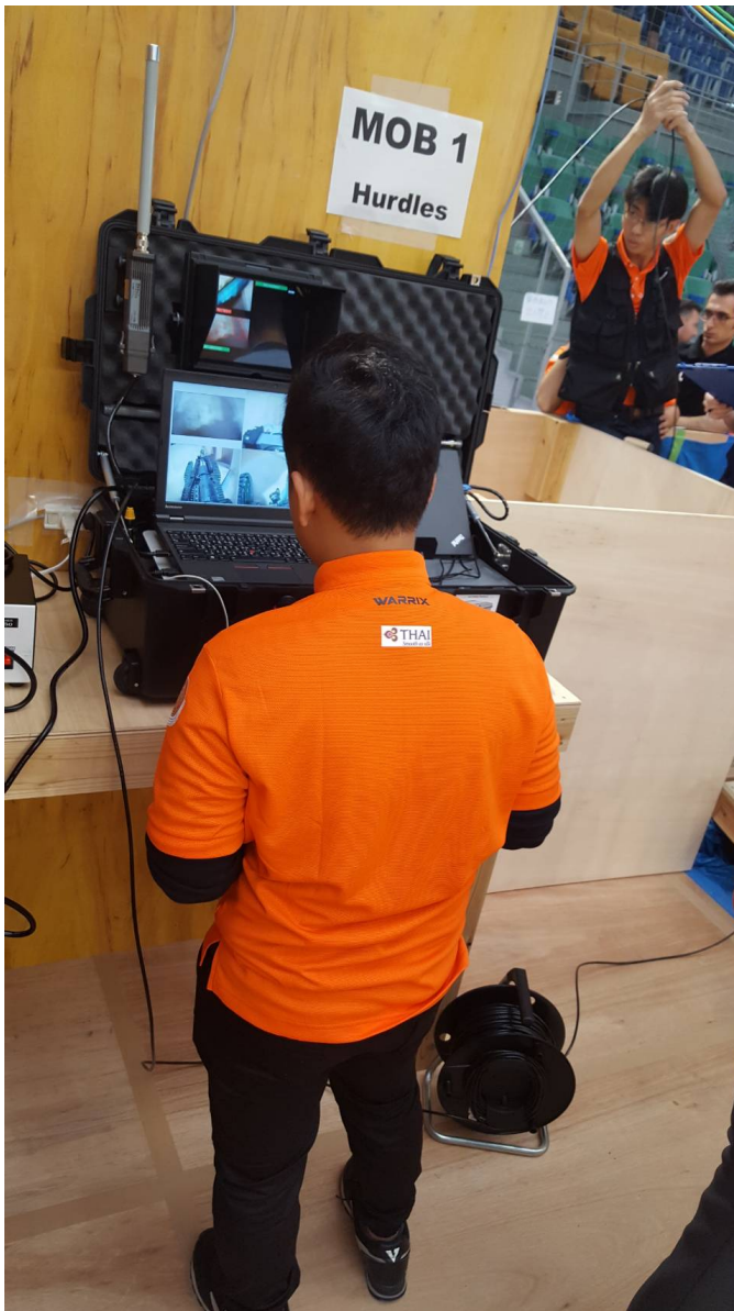
Fig. 10. The operator station used by the driver to remotely control the robot to do the mission from another side.
