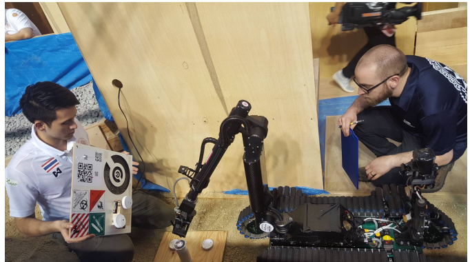
Fig. 4. The robot manipulator arm has a camera and a gripper at the end effector for the readiness test.
