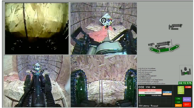
Fig. 8. The operators display illustrated the real-time quad videos' frame and the information of the sensors.
