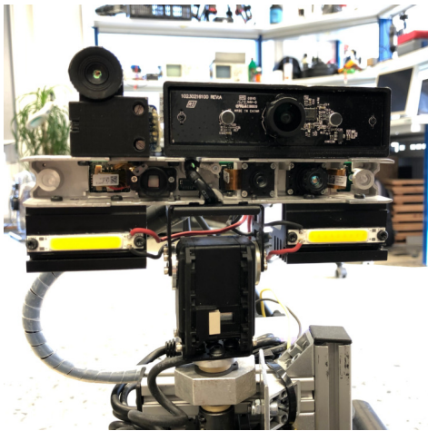
(a) Sensor head with IR-Camera, RGB-Wide-Angle-Camera, 3D Structured-Light-Sensor.
