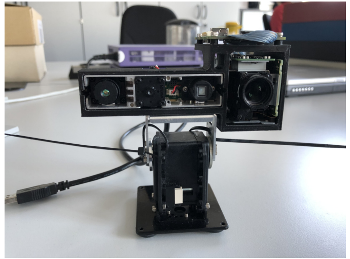
Fig. 6. New Sensor Head. Image shows the status of the new sensor head. SeekThermal device and Basler RGB camera will be added.
