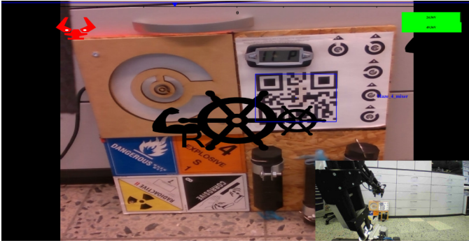
Fig. 7. Head Up Display in Manipulator Mode. Image shows, the GUI is currently in manipulator mode so the picture in picture displays the driver cam, the main camera feed shows the manipulator camera. Two bars represent the current voltage of the batteries, the gripper icon shows, that the manipulator is switched to camera coordinate system.
