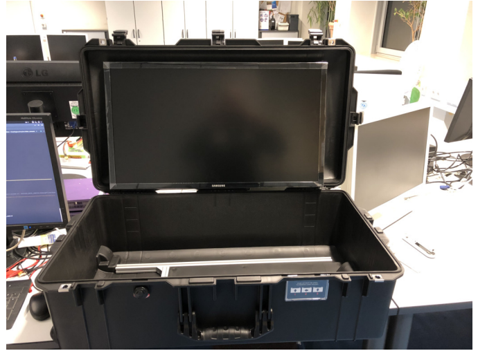
Fig. 8. New operator box. Image shows the Peli Air case with the 28 inch display.
