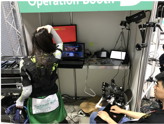
Fig. 3. Demonstrate of visual control set up: HTC vive headset visual system, multi-screen view; and robot manipulation set up: tele-suit control, mannequin control and support operator control
