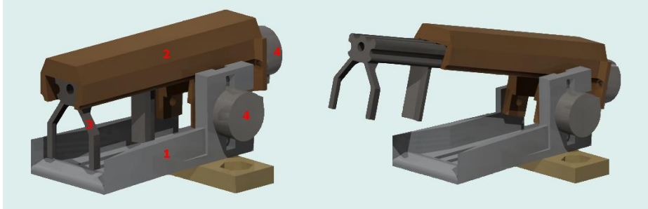
Fig. 1. Gripper Rendering: Basic element with guide rail (1), rail (2), cantilever (3), stepper motors (4)
