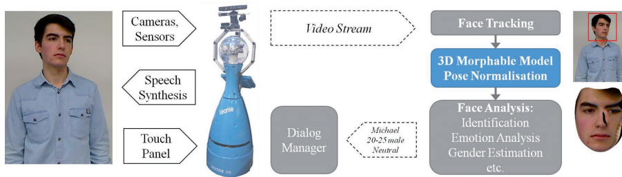
Fig. 1: Pipeline using face recognition and tracking
