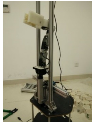
Fig. 7. Elevated arm for flexible height manipulation
