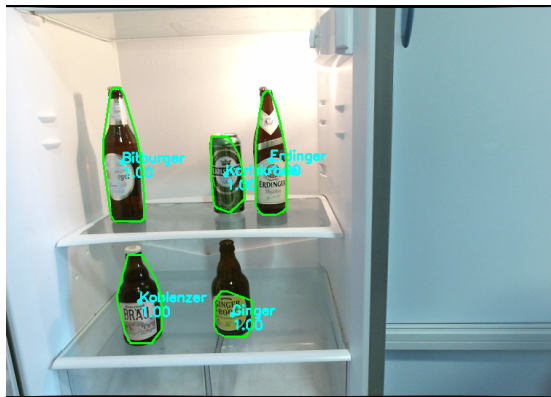
Fig. 3. Prediction result of our home net pixel wise semantic segmentation approach. In this case the net is classifying different kinds of beers.
