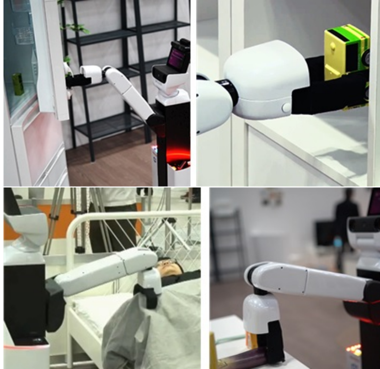
Fig. 2. HSR manipulating various objects at World Robot Summit 2018 competition.
