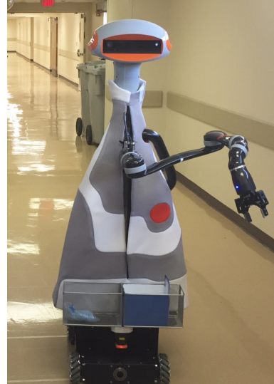
(b) SegBot with mounted Kinova Mico arm.
